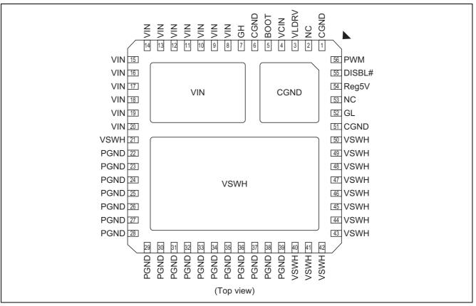
Note: All die-pads (three pads in total) should be soldered to PCB.
