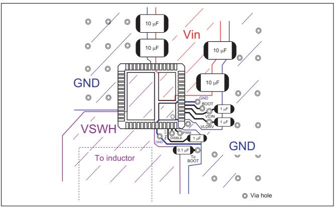
Figure 2 R2J20604NP PCB Layout Example (Top View)
